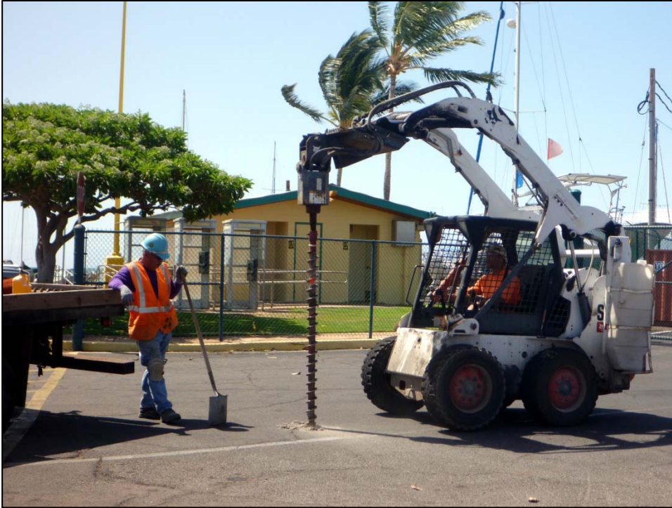
Figure 21. Bobcat with auger attachment.
